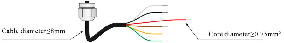
\* Cable diameter  $\leq 8\text{mm}$  (Shown as above picture)
