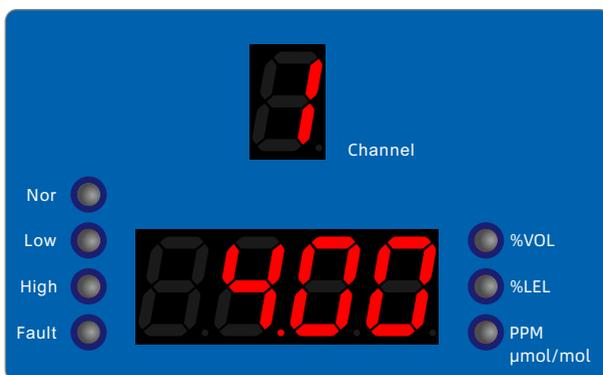
In single-channel mode, the channel displays 1 (currently set channel), and the value below is the current value of the channel.
