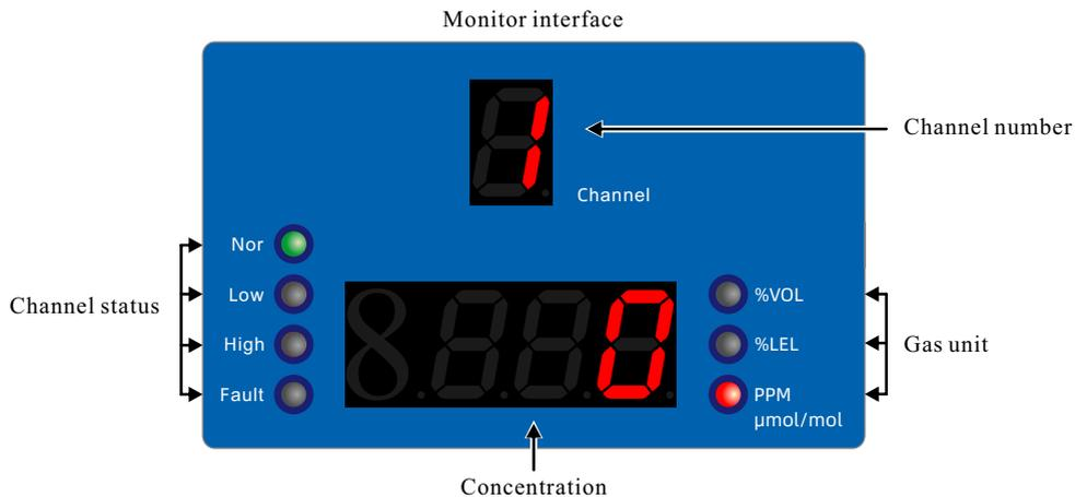
When there is more than 1 channel, the display will automatic cycle display.
