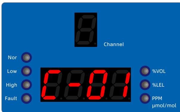
**Single channel mode:** C-01/C-02/C-03/C-04 are optional, each channel needs to be set individually. please follow below rules: zero point  $\leq$  low alarm value < high alarm value < span value.
