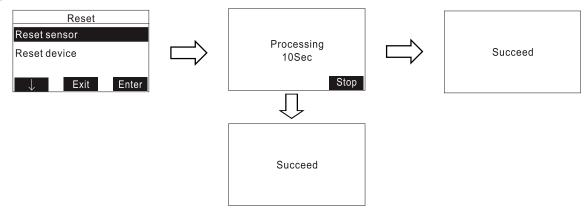
• Press the [Y/+] key to confirm the selection and restore, during which a 10second countdown will be displayed. During the countdown, press the [Y/+] key again to terminate the restoration setting.
