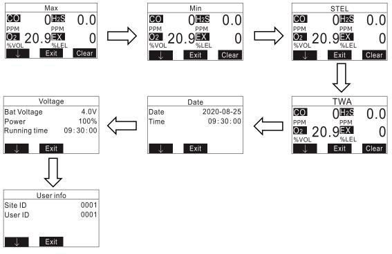
On detection interface, press the [N/-] key to display the following interfaces in sequence.
