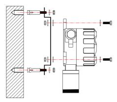
**Note:** The installation location must be well grounded or insulated. Leakage of electricity may cause the detector to work abnormally.
