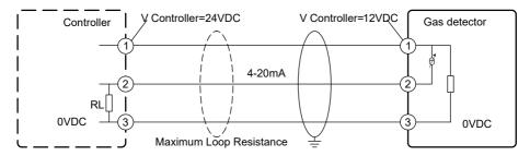
Maximum Loop Impedance: Rloop = (VController – VDetector(min)) / IDetector Calculated according to the above formula.
